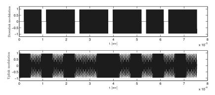
Fig. 2. Example communication signals for ISO/IEC14443-2 type A. Top: Downlink modulation, Bottom: Uplink modulation
