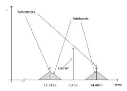
Fig. 5. Spectral image of ISO/IEC 14443 communication
