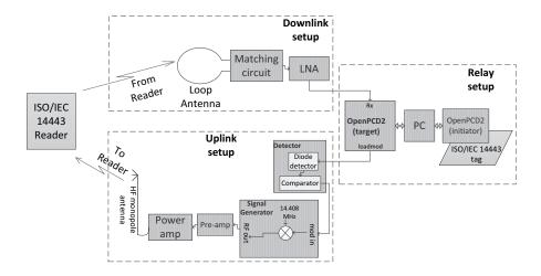
Fig. 3. Block diagram of full range extension system
