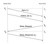
Fig. 1. PTP 2-step message flow. Note the 4 timestamps  $t_1$ ,  $t_2$ ,  $t_3$ ,  $t_4$ : the FOLLOW\_UP and DELAY\_RESP messages carry  $t_1$  and  $t_4$  to the slave.
