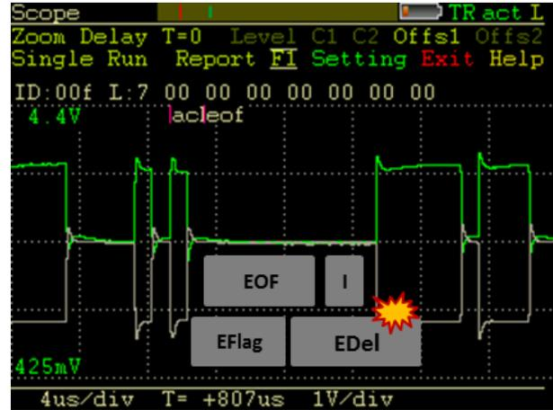
Fig. 6. The minimal gap of 11 bit-time slots, between the 17th silent collision and *Alice's* next  $Dmessage$ . The grey rectangles illustrate both *Eve's* (lower) and *Alice's* (upper) transmitted fields. Notice the interruption in *Eve's* error delimiter (EDel) block, as marked on the right.
