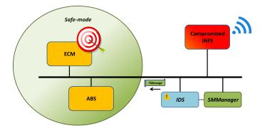
Fig. 2: The system overview. Note that the *SMManager* can be connected directly to the IDS system, or alternatively, get its feedback over the bus.
