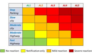
Fig. 5: An example for a 5x5 *Reaction-Matrix*. Note that the rows represent the current *VC* (speed/location), the columns represent the chosen *AL* (1-5), and the colors of the internal blocks represent the chosen *RL* (nothing to severe).
