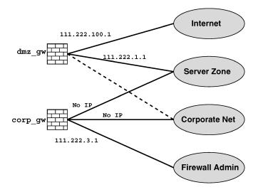
Fig. 4. A bipartite gateway-zone graph  $H = ((G \cup Z), \mathcal{I})$  for the network topology of Figure 3, with interface edges shown as solid lines. *G* consists of two gateways, *Z* consists of four zones. The edges in  $\mathcal{I}$  are labeled by the IP addresses of the interfaces they represent. Adding a third interface to dmz\_gw, whose adjacent zone is the corporate net, would add the dashed line to the gateway-zone graph and create a cycle.
