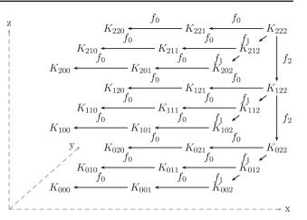
Fig. 3 The hash matrix for m = 3, d = 3. Arrows indicate the key computation sequences
