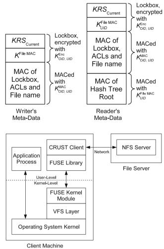
Fig. 6 Architecture of CRUST layered over NFS. Note that NFS is just an example. CRUST can be layered over any file system
