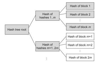
Fig. 2 The hash tree structure, where each internal node has m children. The *grayed* nodes need to be accessed for verifying any block in the range 1...m
