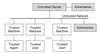
Fig. 1 The CRUST trust model. Untrusted entities are grayed
